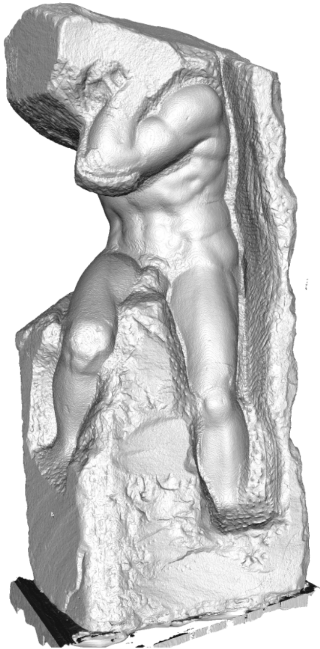
Figure 4.7: Reconstruction of Michelangelo's Atlas with 410 million points (9.15 GB of data) at depth 12 with D4 wavelets took less than 2.5 hours and produced 42.7 million polygons.
